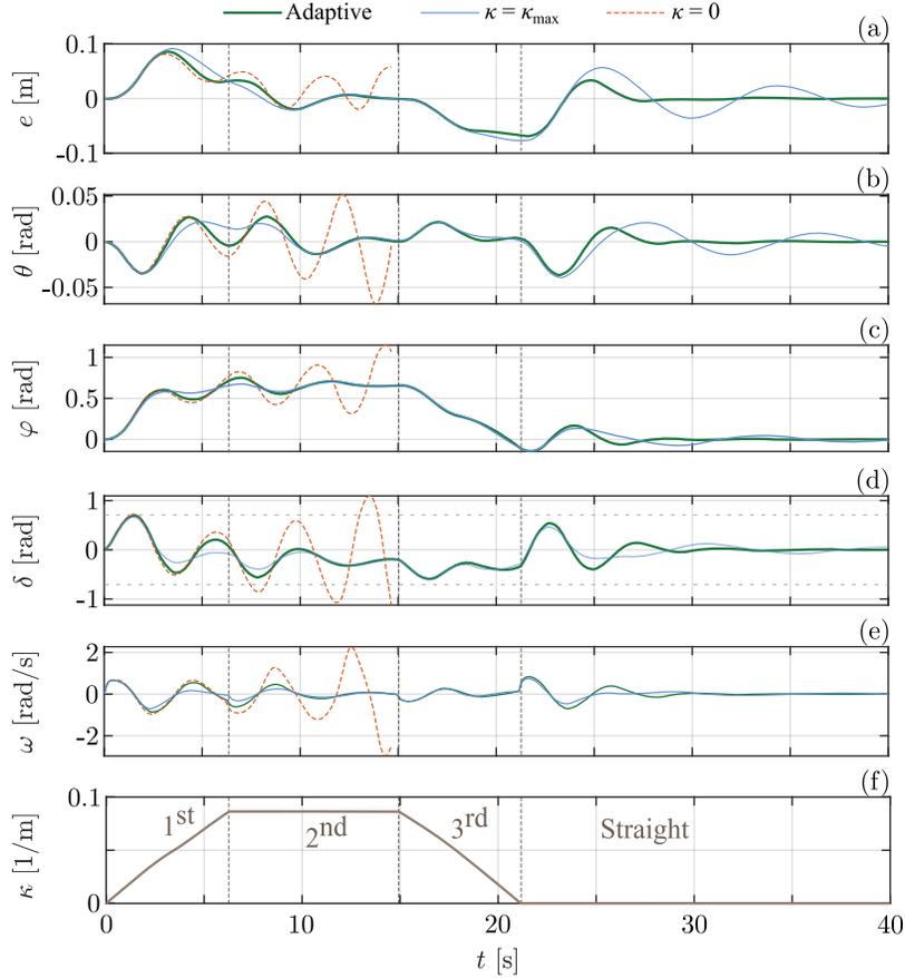
Fig. 3: Simulated time series of the state variables during the 90-degree alley dock (i.e., reversing along a path with varying curvature) with time delay  $\tau = 0.5$  s in order to demonstrate the differences between the three distinct gain tuning methods. The control gain related to the lateral deviation is  $P_e = -5$  rad/m. Vertical dashed lines separate the segments of the path. Horizontal dashed lines in (d) mark the physical limit of the steering angle.
